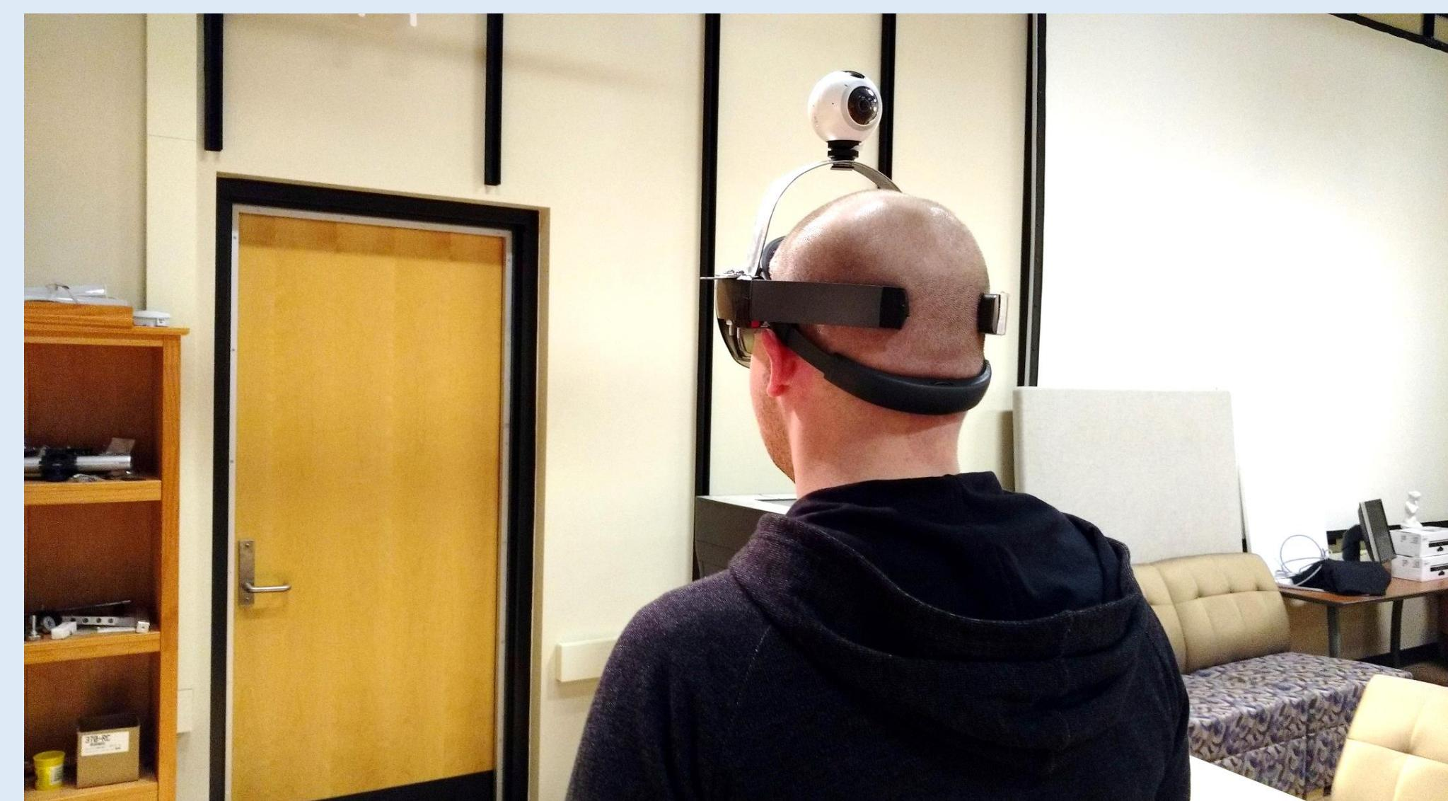
Figure 1: The user walks through the scene while wearing an AR HMD enhanced with a panoramic video camera.
