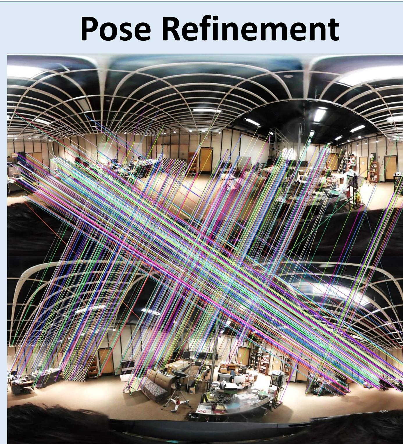
Figure 5: Feature matches between adjacent panoramas, after RANSAC outlier removal, used in bundle adjustment to refine estimated panorama poses are refined via bundle adjustment with pairwise matches.
