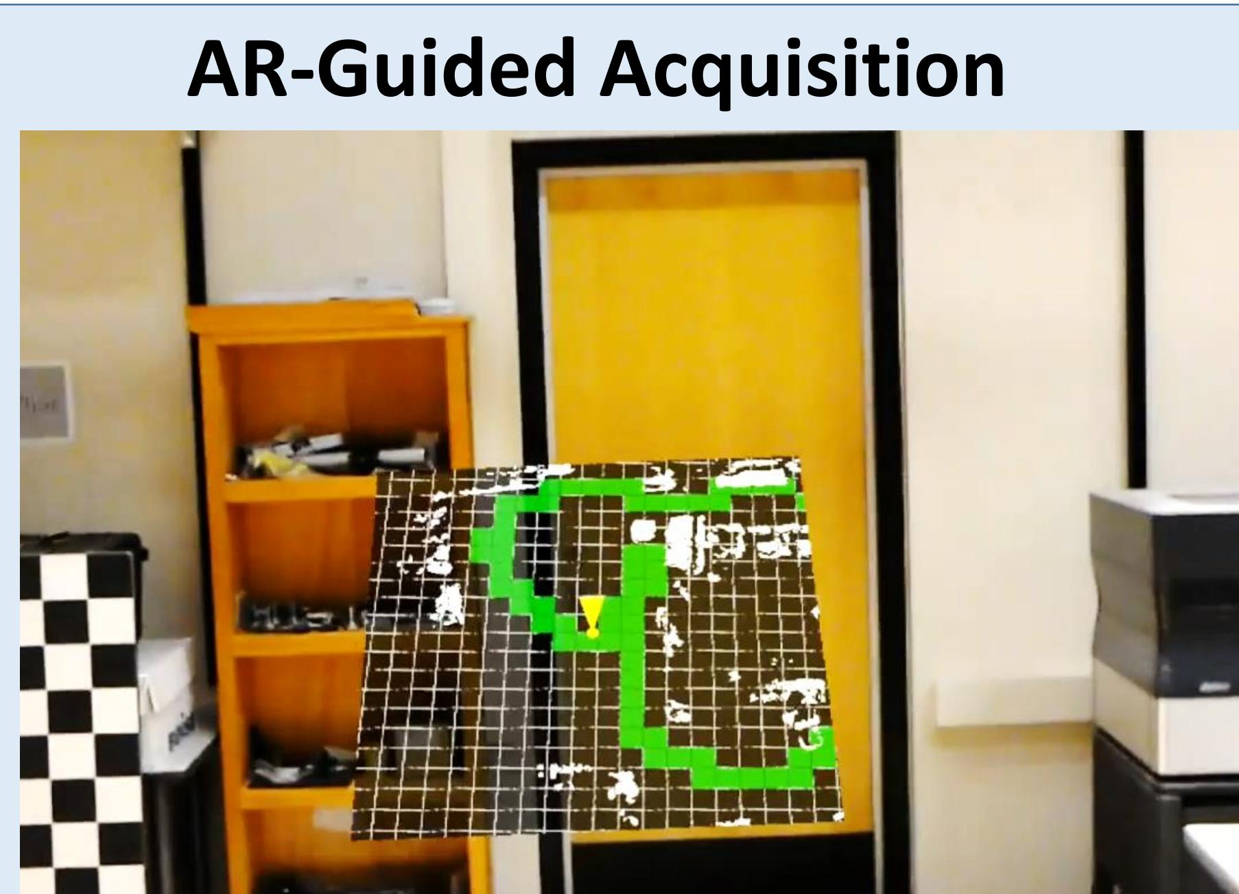
Figure 2: The AR interface shows a 2D grid of a dynamically generated floor plan, which appears as a map floating in front of the user.
