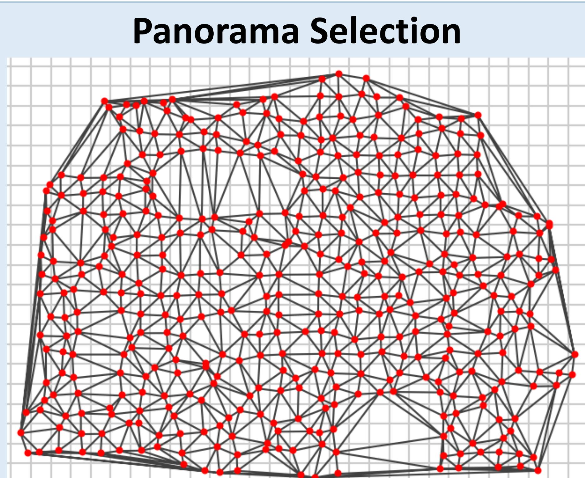
Figure 4: Panoramas (red circles) selected based on estimated AR HMD poses by proximity to traversed grid cell centers and by low rotational velocity. Panorama triplets (gray triangles) defined by Delaunay triangulation.
