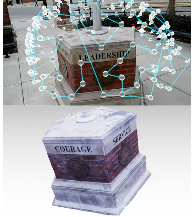
Fig. 5. An example of our AR HMD guided acquisition functioning in an outdoor environment. Top: Suggested views and acquisition path. Bottom: High quality photogrammetric reconstruction.
